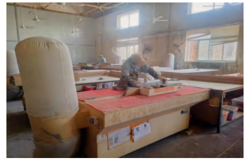
3 手工打磨叶片边部 3.Workers hand sanding for the edge to make sure the edge smooths.
