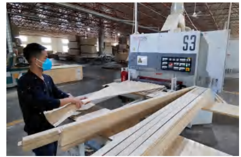
3 手工打磨叶片边部 3.Workers hand sanding for the edge to make sure the edge smooths.
